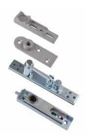
The Briton 2800 Series is designed to accommodate architectural and oversized doors. Pivot sets provide a seamless way of hanging doors, enabling them to swing in either direction. It suits doors with a minimum thickness of 40mm, and a width up to 1100mm.
